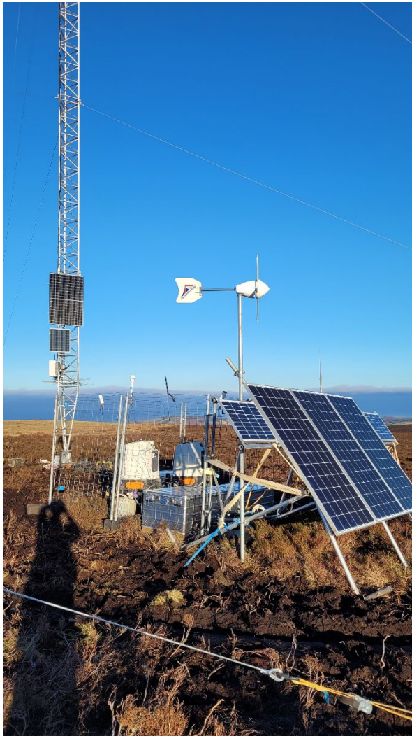
Figure 1: Multi-technology wind measurement campaign set up with ZX 300 wind Lidars, co-located with met mast.
