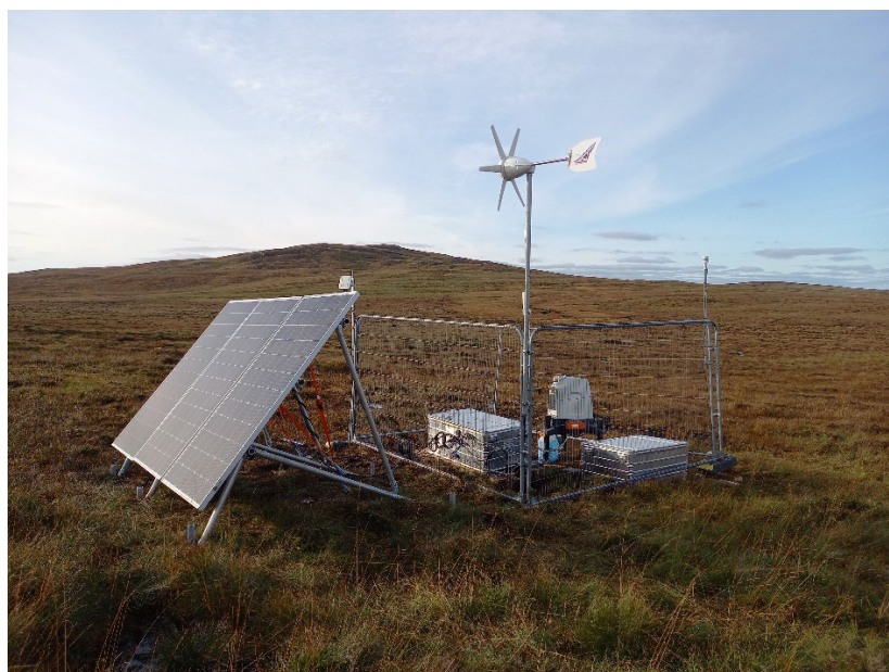
Figure 1: A typical ZX 300 Wind Lidar deployment in terrain that features complex flow characteristics
