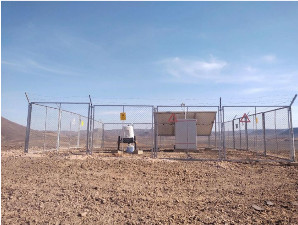
Figure 2: ZX 300 is profiling the wind resource from ground level up to 300m
