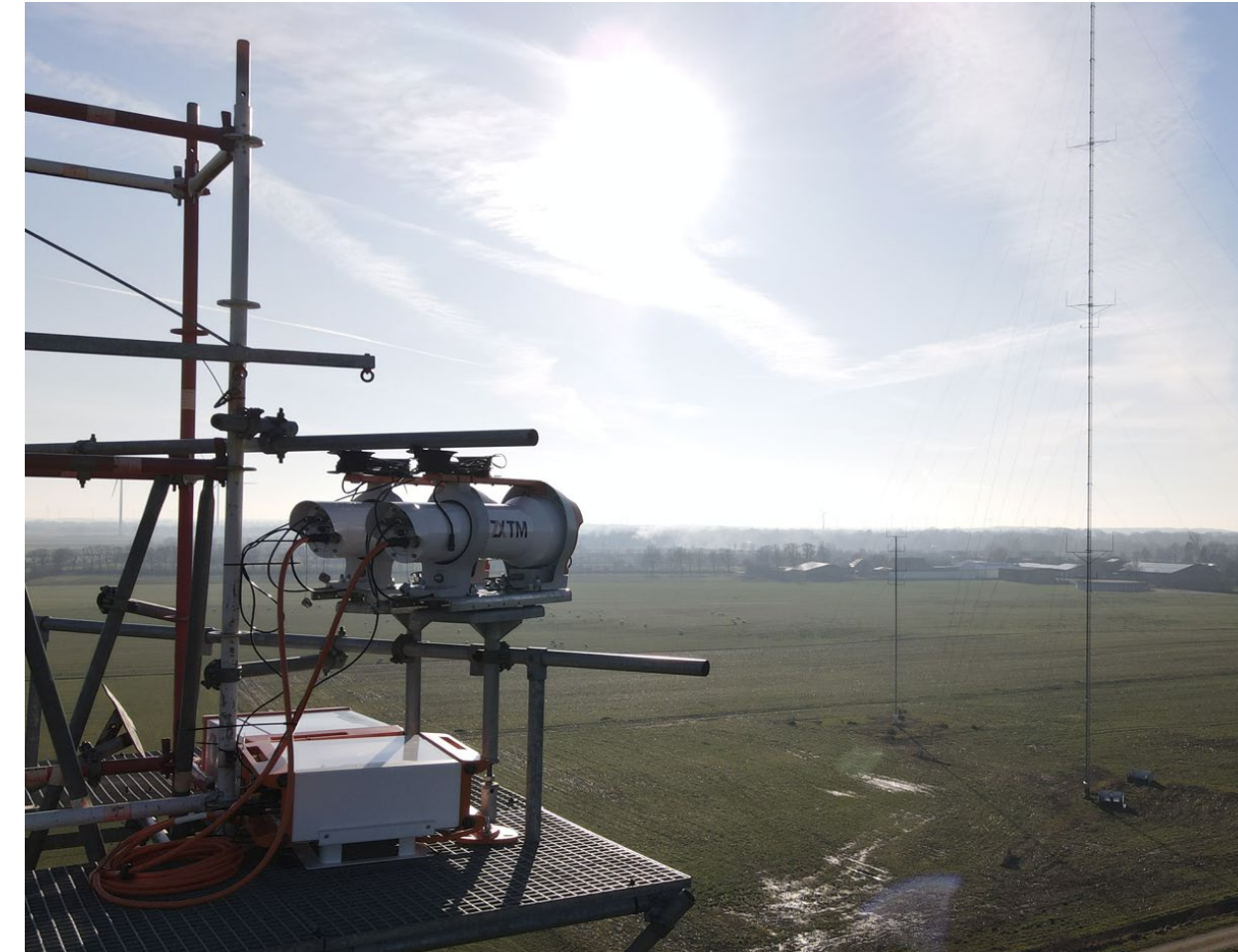
ZX TMs undergoing 50-3 compliant calibration at DNV's Janneby test site, Germany. Image courtesy of DNV.
