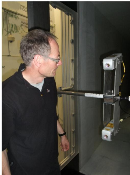
Figure 2 Photograph taken during the experiments showing two lidar transceivers mounted inside the wind tunnel.
