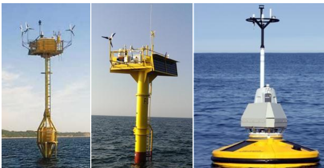
Figure 3: From left to right; SeaRoc’s SeaZephIR tension leg buoy, Babcock’s FORECAST spar buoy and Fugro’s SeaWatch wave buoy.
