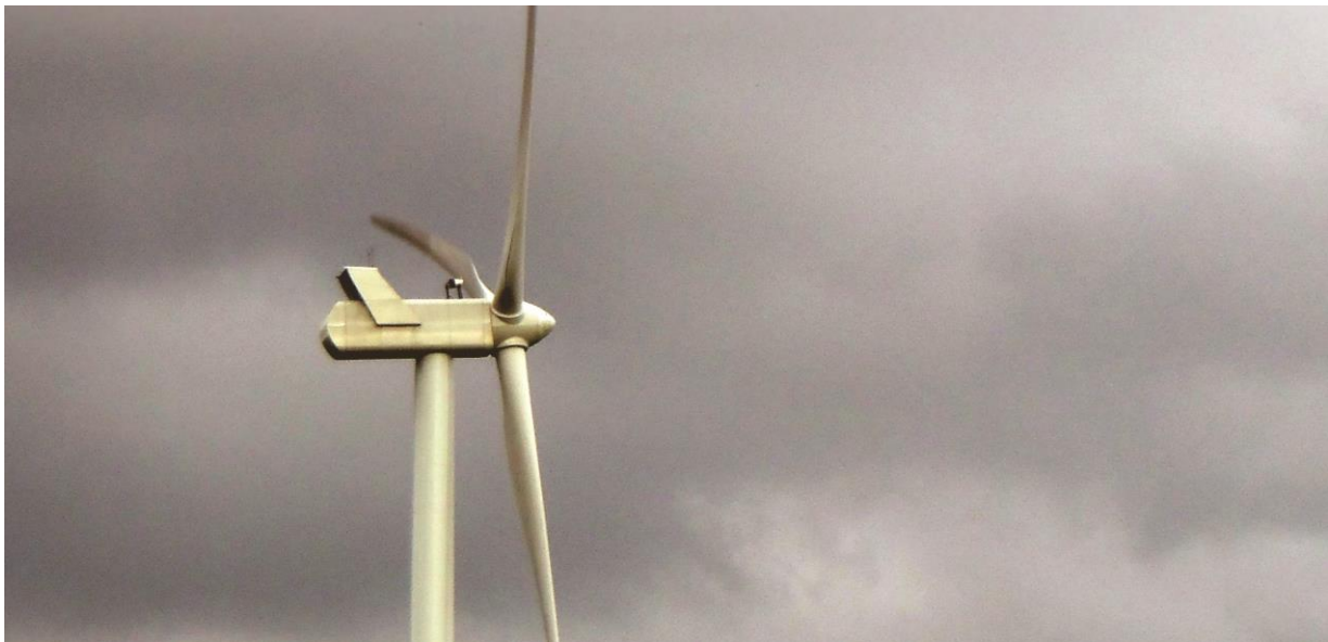
Figure 5: ZepHIR DM installed on a Vestas wind turbine with RES
