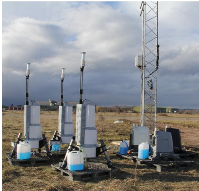
Figure 3 : ZephIR Siting at Mast Base. ZephIR 150 (left) and ZephIR 300 (right).
