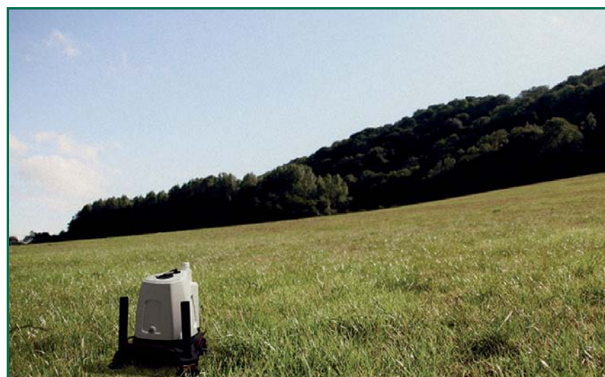
Figure 1. ZephIR 300 deployed in a complex flow environment, using Natural Power's dynamics™ for data conversion
