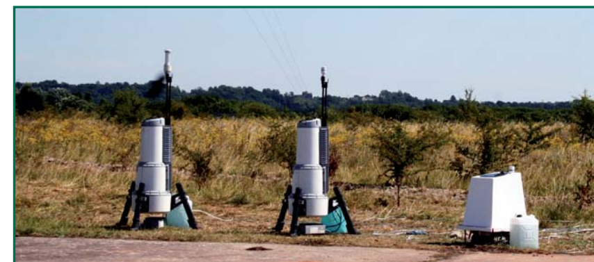
Figure 2. Two ZephIR reference systems providing side-by-side correlations and ZephIR 300 prototype during the 18-month development and validation period
