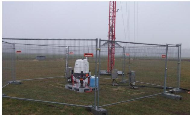
**Figure 1: ZephIR 300 deployed at Test Site Lelystad during its verification.**
