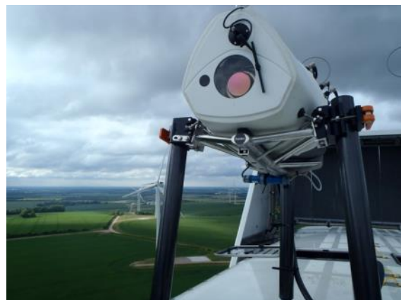
Figure 1: ZephIR DM in operation on Vestas V90 turbine.
