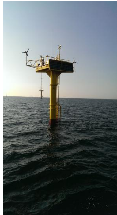
Figure 1: Babcock's low-motion spar buoy with ZephIR 300 visible
