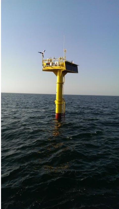
Figure 2: General view of the spar buoy with ZephIR 300 visible in left corner.
